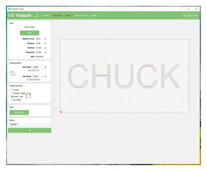
By default Inside / Left is selected. Click the bullet for Pocket under Offset Direction. At the top under tool make sure you have #201 showing, if not Click Edit and in the tool pull down find the #201 tool and click OK to select it. Then move to Name and Type "Pocket Lettering". Your screen will look similar to the screen shown in the image below.
