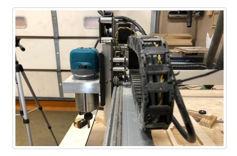
Solution: Adjust the drag chain so it is running perpendicular to the X-axis rail. You can even cheat this so it's running away from the rail towards the back slightly.
