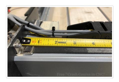
Solution: Adjust the end of the drag chain to be further away from the Y-Axis left plate.
